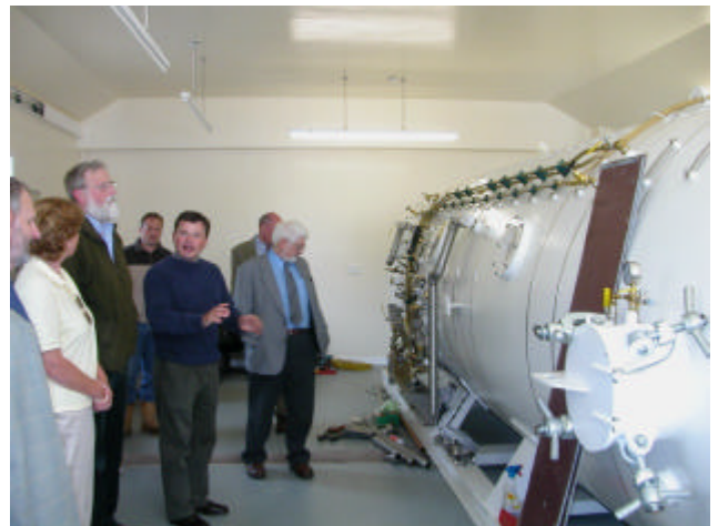
The new recompression chamber for divers
